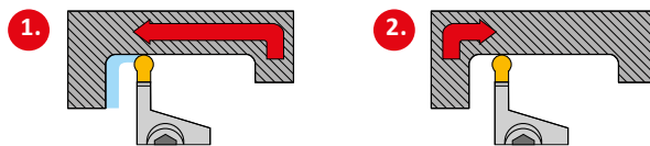
Finishing of contour (insert with round cutting edge)
